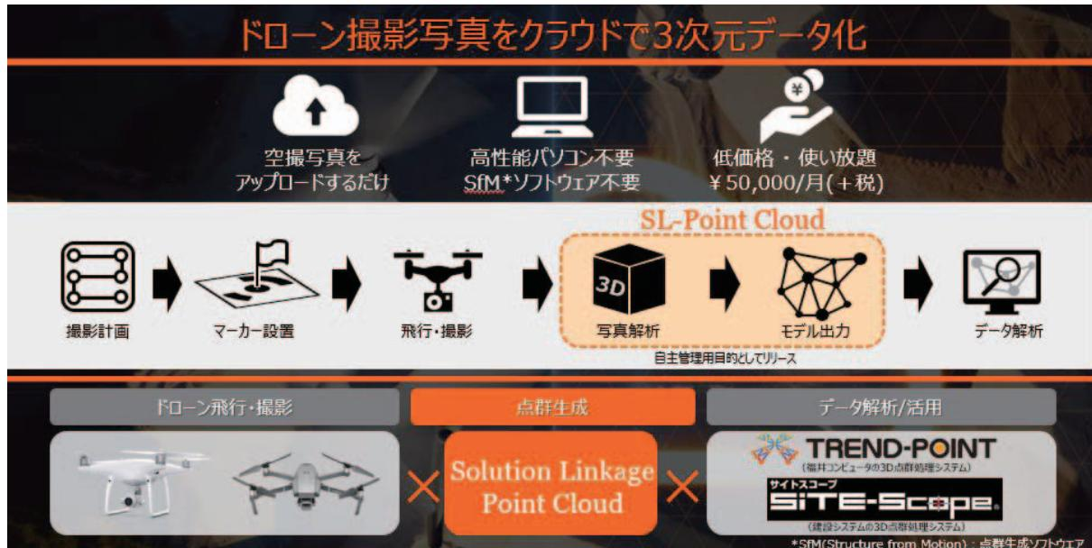
図6 Solution Linkage Point Cloud 概要
